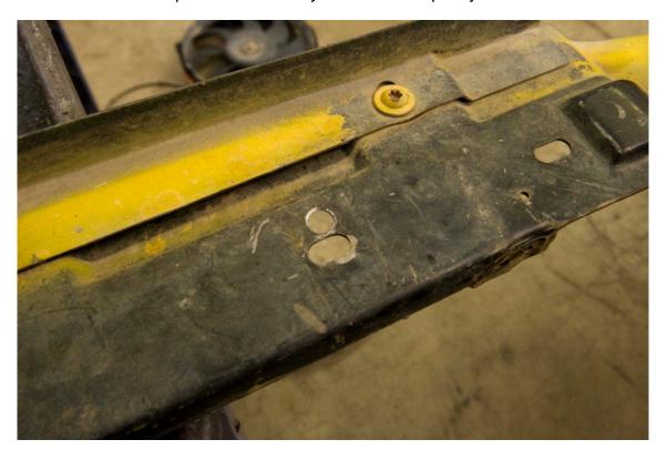
Slide the fan assembly over the radiator, and then re install the radiator support panel. Making sure the rubber mounting brackets are in the re drilled holes.
