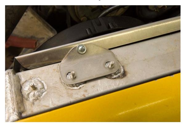
Replace radiator rubber mount and tighten nuts.
