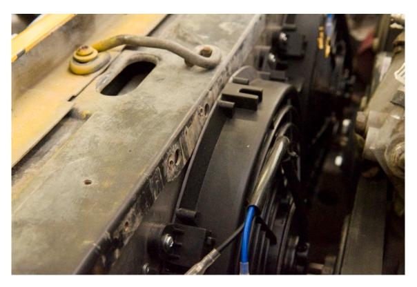
Secure the bottom of the fan shroud with included self tapping screws.
