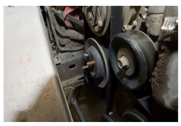
Remove the radiator support panel, and set aside. Remove the radiator rubber mounts and slide fan kit mounting tabs over screws.
