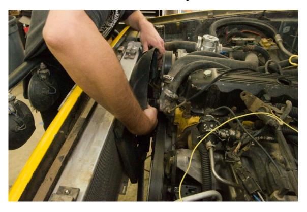
Replace the mechanical fan studs with the provided bolts. Failure to replace studs will void any fan warranty.
