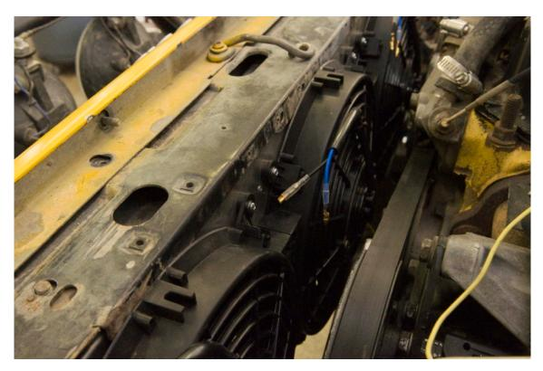
Notice how the radiator support slides between the fan and the shroud.
