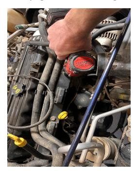
Step 3 (optional): Good time for a tune up! We recommend using OE plugs, the part # and gap information can be found on your engine Catalyst under the hood
