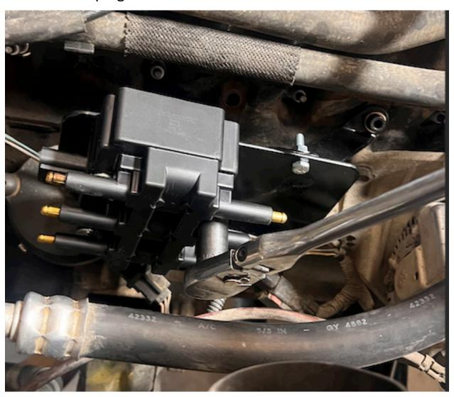
**Step 10:** Install the provided extension harness to plug into the OEM ignition rail plug and the other end into the new coil pack.
