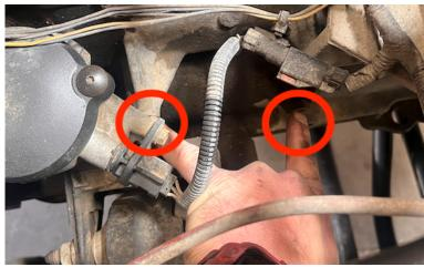
**Step 6:** Using the 14mm socket, tighten down the mounting bolts on the bottom of the bracket into the block.
