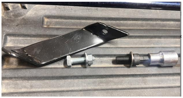
**Step 8:** Install the support brace with the flat edge towards the coil bracket, and round edge towards engine. 1/4-20 bolt goes into the bracket, the cap screw goes into the block in the OE ignition rail mounting hole.
